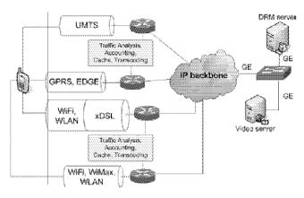
Figure 5 The generic scheme of the media streaming testbed [25]
