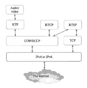
Figure 7 Streaming protocol architecture
